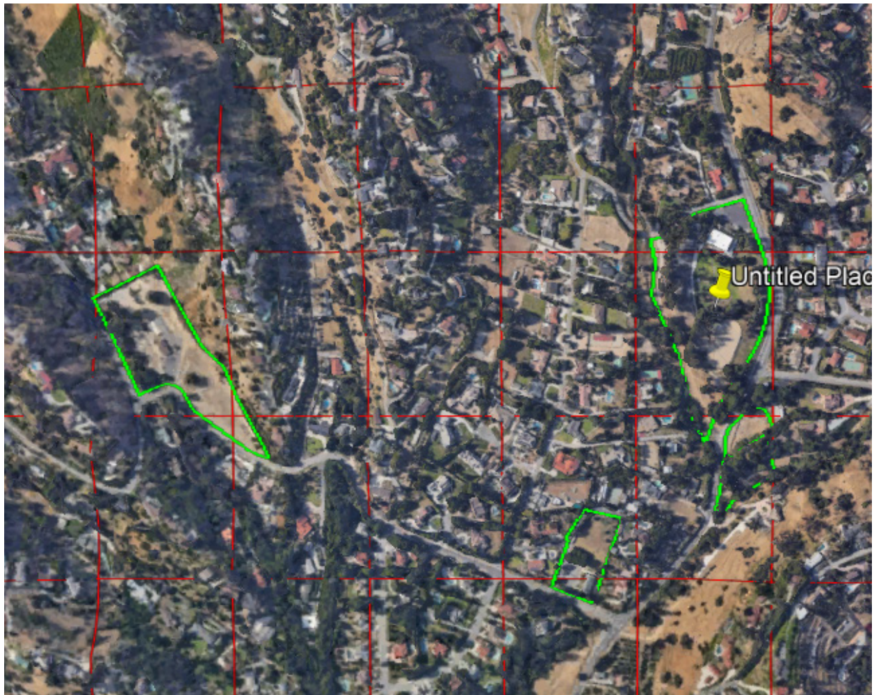
Figure 23: Example of highlighted Landvision parcel data (bright green polygons) showing areas that are zoned for retail or public use. CT scanning can focus on these areas and ignore other areas, including those zoned for single family homes.
