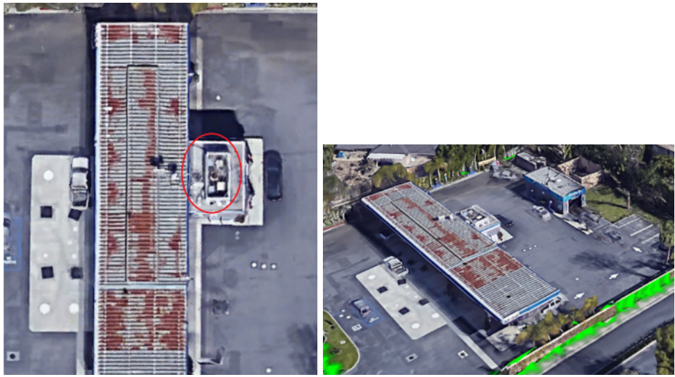
Figure 8: Could there be a CT in this side structure (red circle)? Oblique views show us this is a carwash and thus nothing to cool (no need for a CT).
