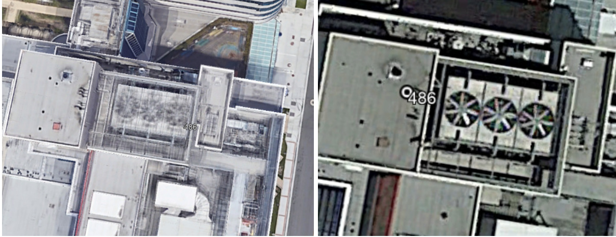
Figure 14: Use non-3D view in Google Earth if 3D renderings are unclear. Google Earth's default 3D view can help provide seamless oblique views, but can also obscure details. Left image shows a hospital with CTs that are easily missed because the fans are blurred. Right image shows the view of same area after switching off 3D view, revealing clearly that these are three CTs with distinctive fans.
