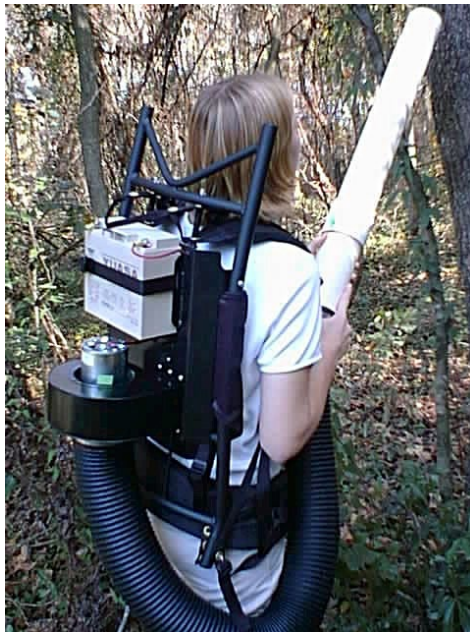
Figure 8: Modified CDC Backpack Aspirator.
