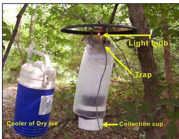
Figure 7: CDC Trap as Set by Fairfax County Health Department, VA.
