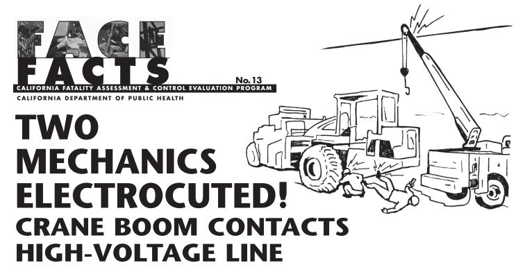
In a recent incident, two mechanics, 18-year-old David K.\*, and 40-year-old Shawn P.\*, died when the truck-mounted crane they were using touched an overhead power line. They had been using the crane to repair a heavy equipment scraper. The boom of the crane touched the high-voltage line. The electrical current passed down the boom to David and Shawn.
