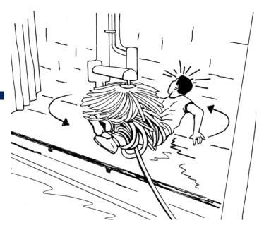
A twenty-three-year-old Hispanic car wash attendant, Manuel P.\*, died while cleaning the floor inside a car wash. Manuel used a hose to clean the floor. He turned on the wash equipment to have more pressure in the hose. As Manuel was spraying the floor, the hose caught in one of the turning brushes. Manuel was pulled into the brush and thrown against the wall.
