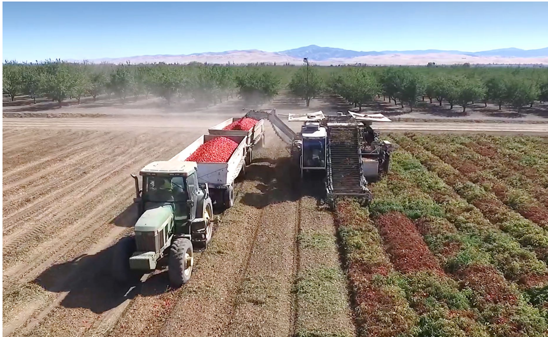
Exhibit 2. A tomato harvester (on right) during the harvesting process. Photo courtesy Westside Equipment.
