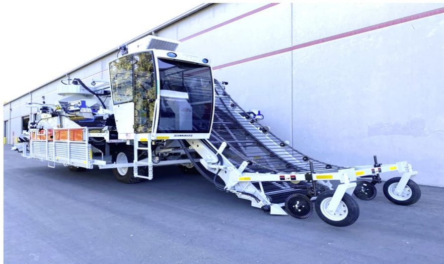
Exhibit 1. A tomato harvester machine (similar model, not actual used in incident). Photo courtesy Westside Equipment.
