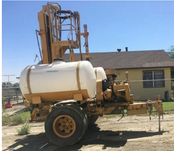
Exhibit 2. Spray rig with open raised aerial bucket similar to the one the victim was in at the time of the incident.
