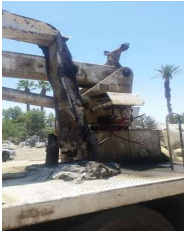
Exhibit 2. The melted bucket that held the victims when they made contact with the high voltage electrical line.
