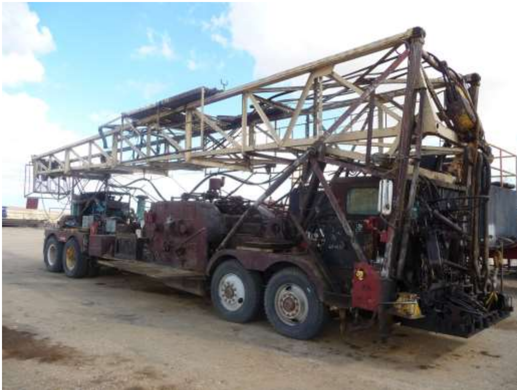
Exhibit 1. The mobile oil well servicing rig involved in the incident.
