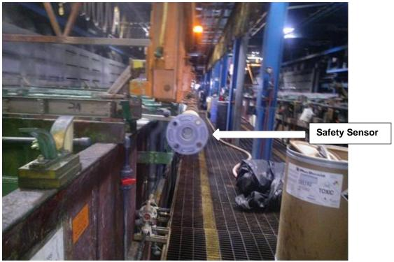
Exhibit 4. The safety sensor device designed to stop the hoist movement when contact is made.
