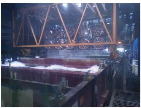
Exhibit 3. The computer controlled hoist with an attached cage for the wheels.
