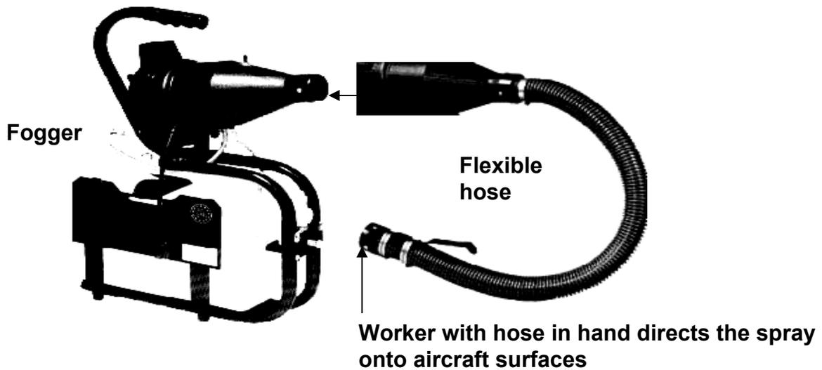
**Figure 1. Pesticide spray-mist fogger.** The fogger holds three gallons (11.4 L) of pesticide solution. *A flexible hose was attached to the nozzle of the fogger. Two workers each pulled a fogger through the aircraft on a wheeled cart while holding the flexible hose and directing the spray onto all surfaces and the overhead storage bins. The pesticide solution was dispensed through the flexible hose as an aerosol with a particle size in the 5-40 micron range.*
