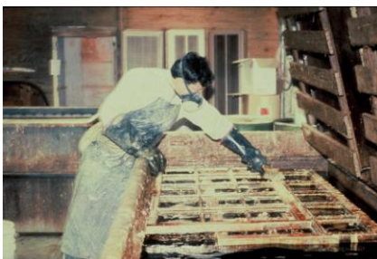
A worker removing paint from a window frame in a dip tank containing a MeCl-based stripper.
