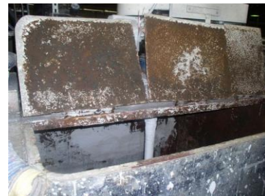
The opening of a paint mixing tank in which a worker died while using a MeCl-containing paint stripper.
