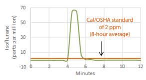
This graph shows isoflurane levels while technicians roll a dog over. The peak on the graph occurred when the endotracheal tube was disconnected to reposition the animal while gas was still flowing. If high exposures like this occurred multiple times during a shift, workers could be exposed over the legal limit.
