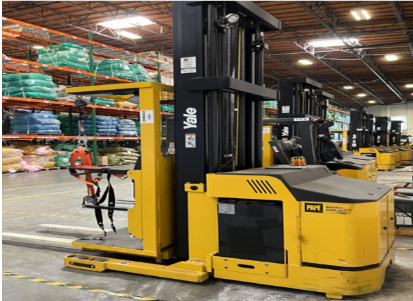
Exhibit 3: The order picker forklift involved in the incident. The arrow indicates where the self-retracting lanyard connected to the body harness was hooked to the forklift. Photo courtesy of CA/FACE program.
