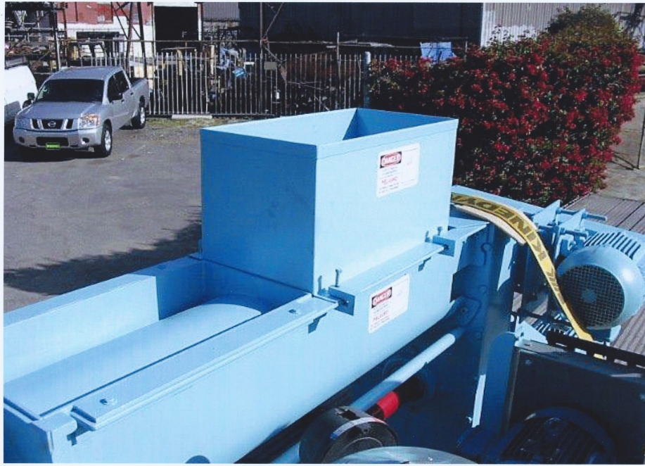
Exhibit 3. A pug mill with safety chute covering the auger blades.
