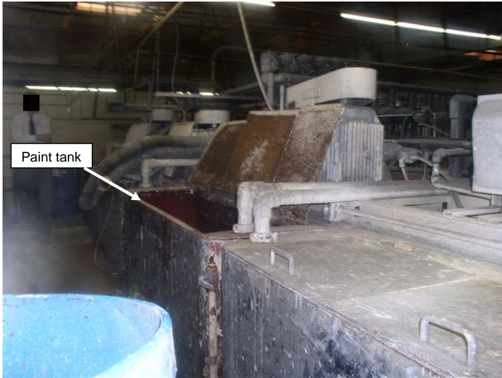
Exhibit 2. The paint tank the victim was cleaning.
