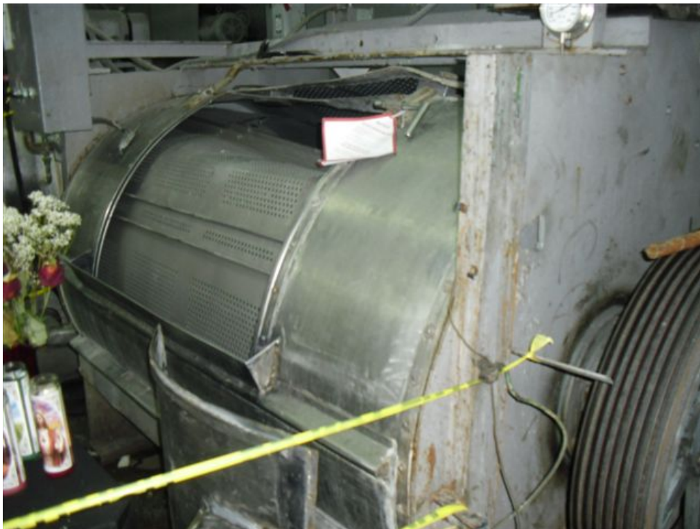
Exhibit 3. The industrial washing machine with the sliding door open, exposing the inner rotating barrel.
