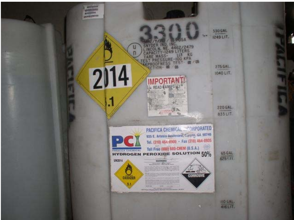
Exhibit 3. The labeling on the hydrogen peroxide tank.
