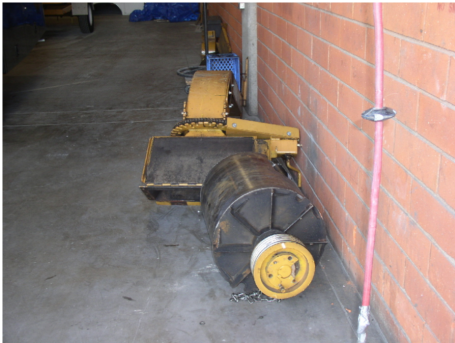
Exhibit 3. The discharge chute and drum that were removed from the brush chipper during the initial investigation.
