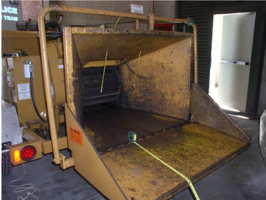
Exhibit 4. The in-feed chute and shroud that feeds the tree limbs into the feed wheel.
