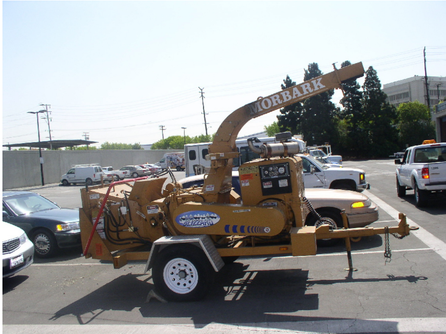
Exhibit 6. A fully assembled brush chipper similar to the one involved in the incident.
