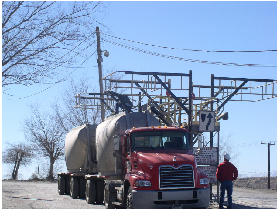
Exhibit 5. An employee utilizing fall protection and the guardrail as he closes the lid on top of the tanker trailer.
