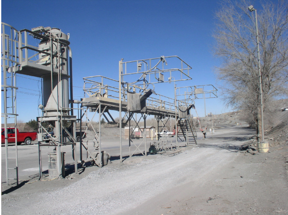
Exhibit 1. The catwalk used by truck drivers to gain access to the top of their tank trailers.
