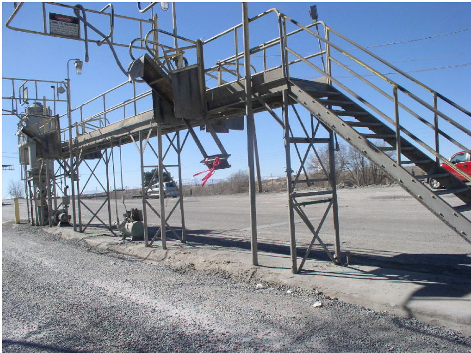
Exhibit 2. The stairs used to gain access to the catwalk and the weighted gangway.
