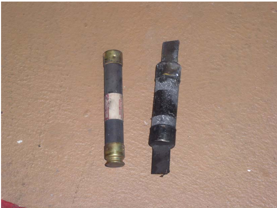
Exhibit 3. A picture of fuses involved in the incident. The fuse on the left was a 30 amp barrel-type fuse that the victim removed from the panel. The fuse on the right was a blade-type fuse the victim tried to use to replace the fuse on the left.
