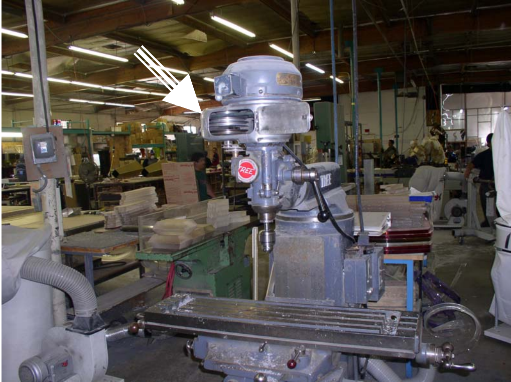
Exhibit 2. A picture of the vertical milling machine involved in the incident with the arrow pointing to the open safety cover for the belt drive.
