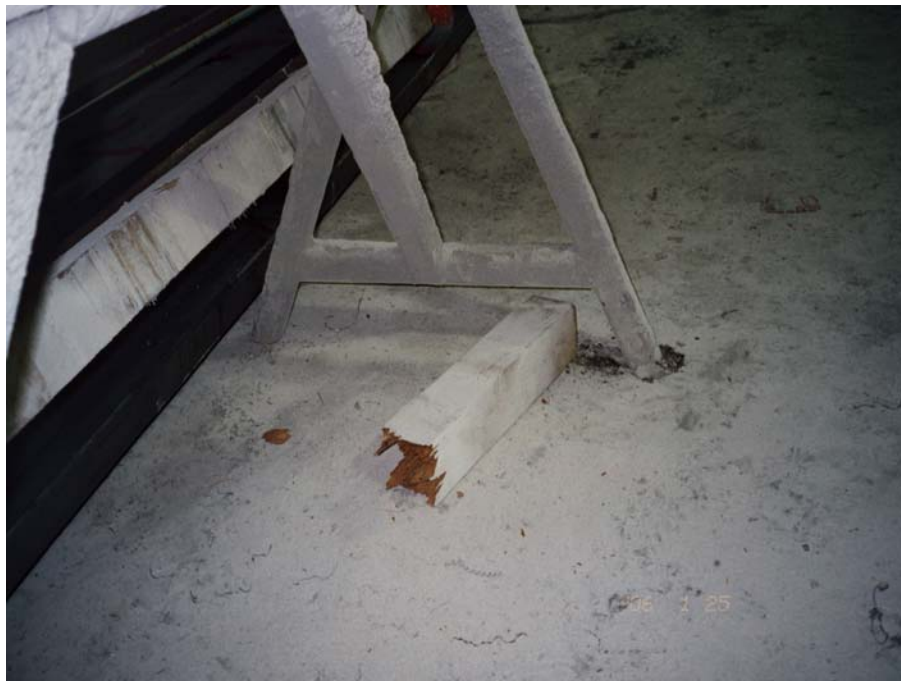
Exhibit 7. A picture of a piece of the wooden beam that broke under the weight of the steel frame.
