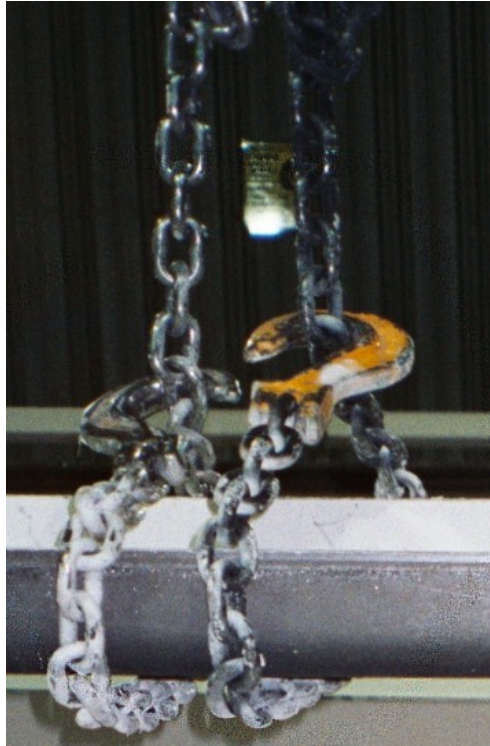
Exhibit 4. A picture of a chain sling in a choker hitch position that was used to pick up the steel frame.
