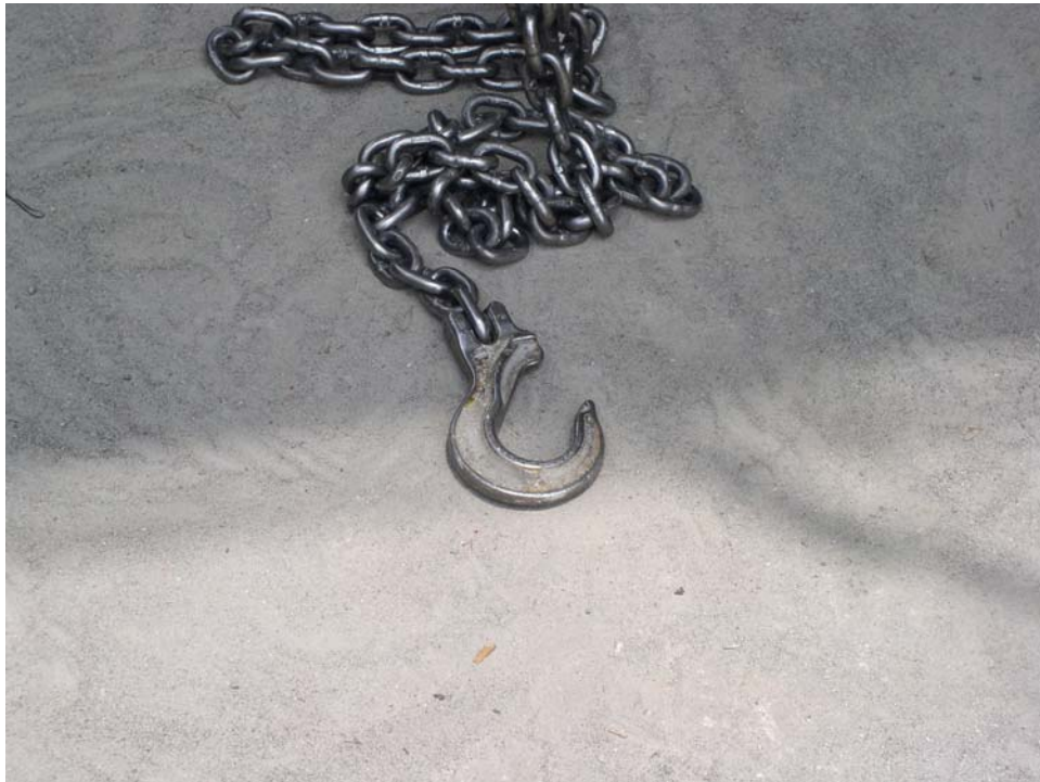
Exhibit 3. A picture of the chain sling that was used to lift the steel frame from a horizontal position to a vertical position.
