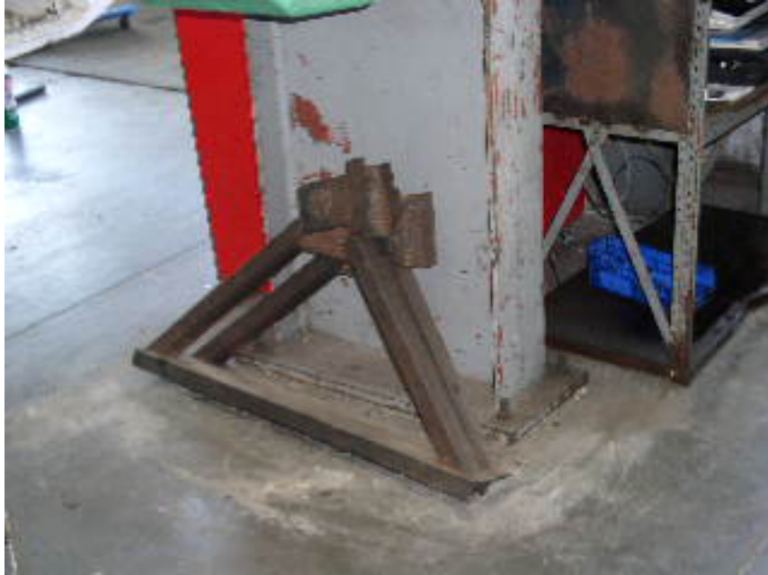
Exhibit 4: A picture of the safety jack stands used to support the bed of a roll-off trash truck in the raised position.
