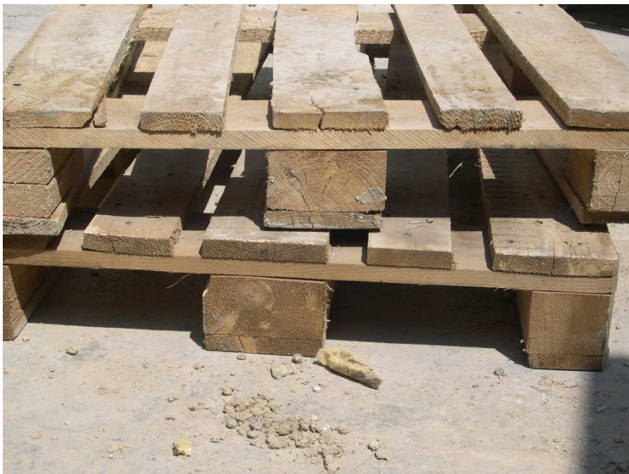
Exhibit 4. This type of pallet is strong enough to support stacked concrete and stone castings.
