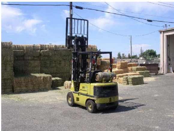
Exhibit 3. The forklift mast in the raised position.
