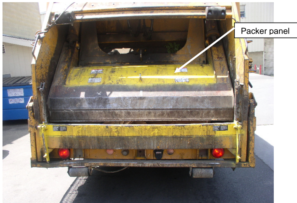
Exhibit #4. A picture of a rear loading trash truck, similar to the one involved in the incident, with the packer panel in the position when it struck the victim who was reaching into the hopper.
