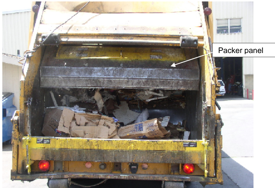
Exhibit #3. A picture of a rear loading trash truck, similar to the one involved in the incident, with the packer panel at the beginning of its cycle.
