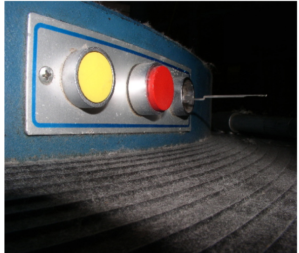
Exhibit 3: The control buttons with a needle stuck in the green button.
