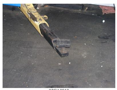
03CA0010 Exhibit #3 A picture of the automotive lift arm with the adjustable pad on the end.
