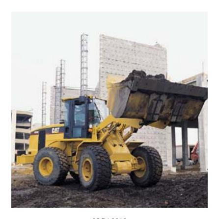
$\begin{array}{c} 02 CA0010 \\ Exhibit \, \#1 \end{array}$  Picture of an articulating front-end loader similar to the one involved in the incident.
