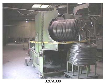
02CA009 Exhibit #2 View of the wire pulling machine and the wire holding device.
