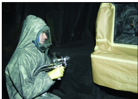
Photo: Worker applying spray-on polyurethane truck bed liner
