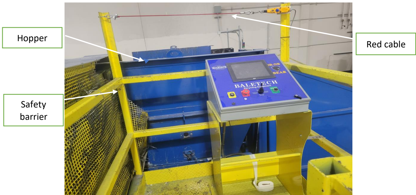
Exhibit 6. The yellow barrier around the control panel to prevent access to the hopper. The red cable was added after the incident occurred. Photo by CA/FACE program.
