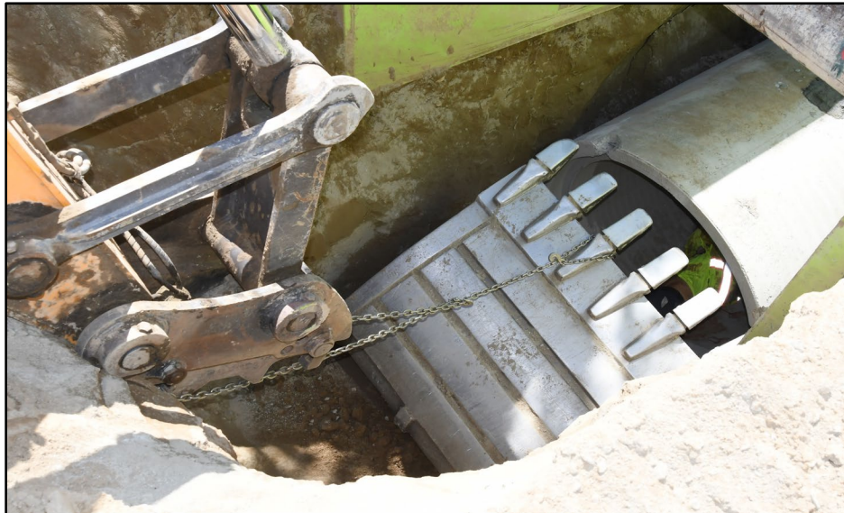
Exhibit 5. View into the trench where the victim was standing and where the bucket detached from the quick coupler. Photo courtesy of police department.
