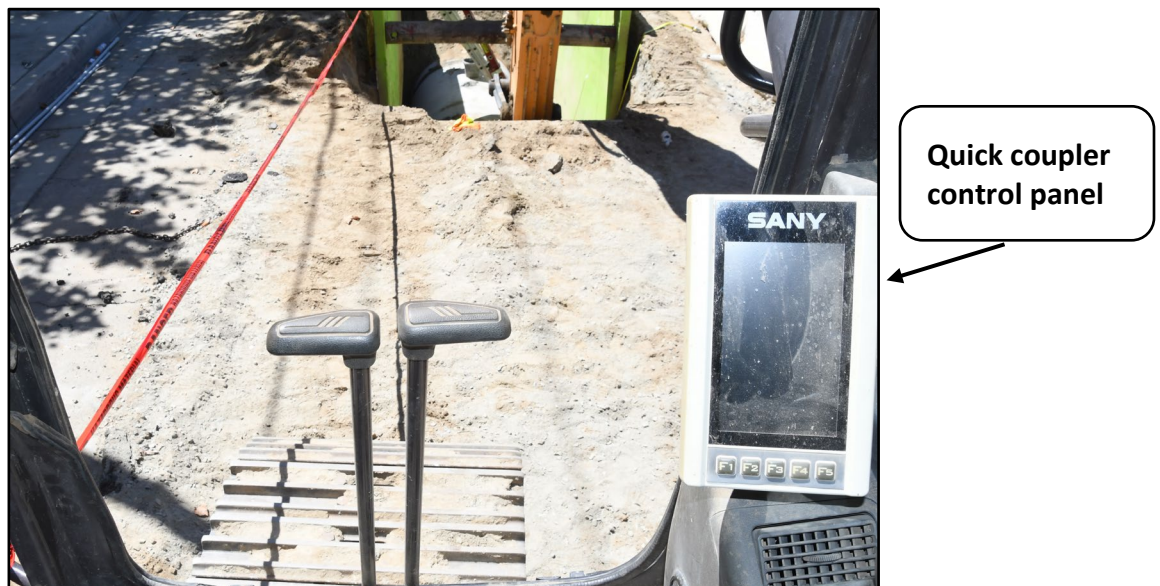
Exhibit 4. The control panel used to operate the quick disconnect. Photo courtesy of police department.
