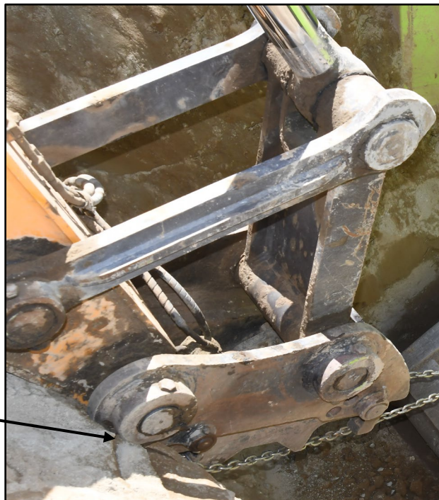
Exhibit 2. A close-up of the quick coupler in this incident. Photo courtesy of police department.
