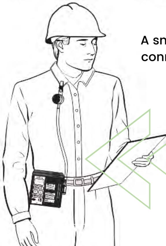
**A small battery-operated pump is connected by a tube to a sampler designed to collect dust.**
