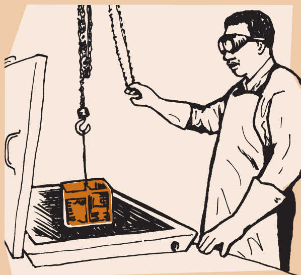
1-BP is used in vapor degreasing to clean metal parts
