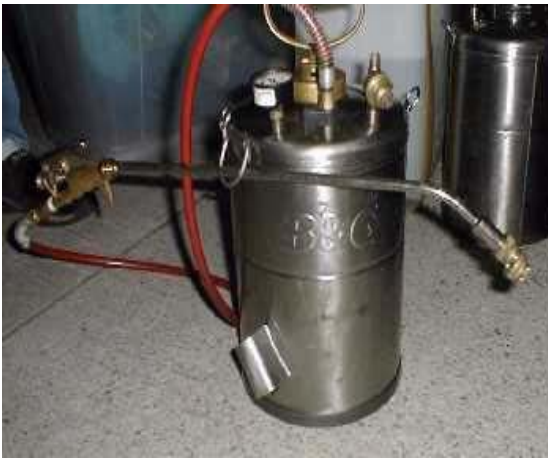
Figure 2. Hand-held sprayer. The sprayer applied a pesticide mist at the rate of 6.4 ounces per minute to the galleys, crew rest area, bathrooms, cockpit, carpet, and cargo hold.
