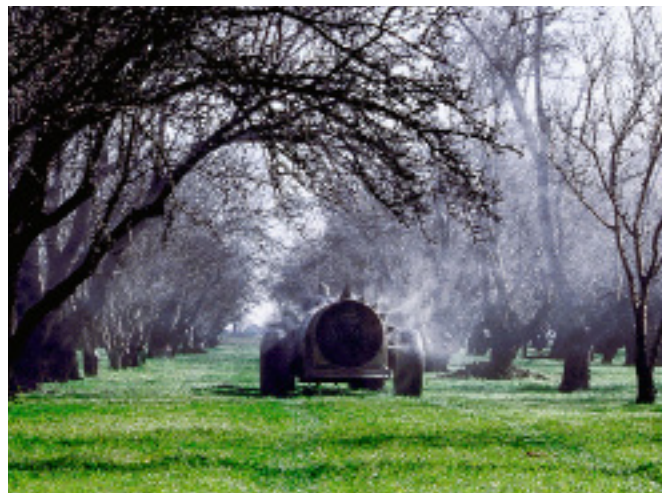
An airblast sprayer applies pesticides to an orchard. Copyright © 2005 The Regents of the University of California. Used by permission.
