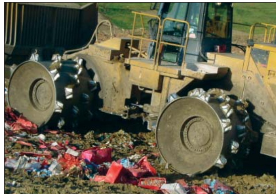
Figure 29. Compacting treated medical waste at landfill
