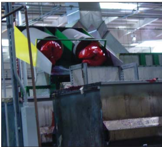
Figure 19. Waste tipped into autoclave bin
